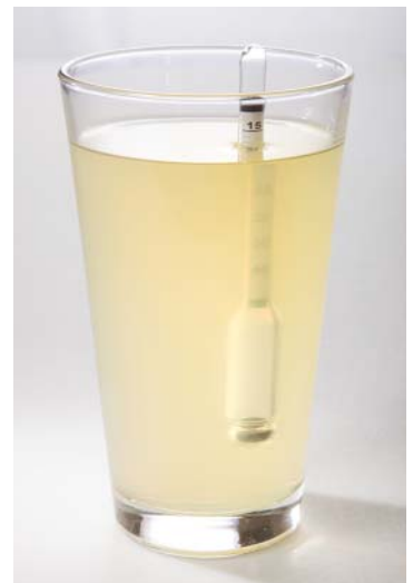
Testing a sorbet mix with a hydrometer.
